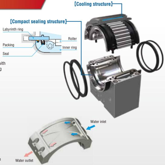
■ ■ ■ Measures for ultralow-speed rotation and water / mill-scale intrusion
