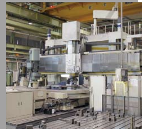
Large five-axis milling machine 大型5面加工機
