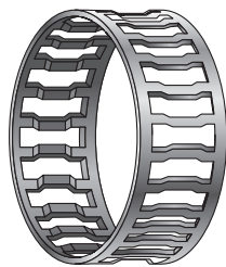
Fig. B4-13. Steel cage
