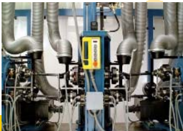
BEHEM CV-joint test bench, plant Hagen
