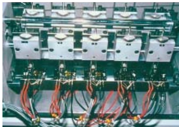
Test of electrical contacts in model switches.
